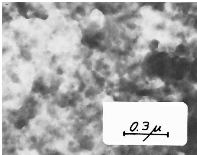
Fig. 5. PVC/P(B-co-AN) cast film. Electron micrograph of unstained sample.
